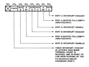
Figure 4. Status Register Bit Assignment
